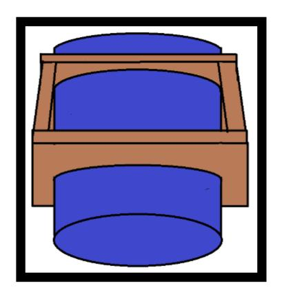
Add the 2  $\times$  10s to the barrel and lock down the base of the barrel with some 2  $\times$  4s. Voila!
