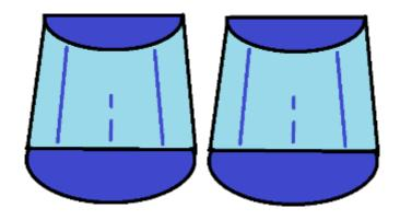
Cut the barrels lengthwise, as shown here
