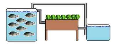
The CHIFT system. The dark gray pipes lead to the sump pit. The light gray pipe transport water back to the holding tank.
