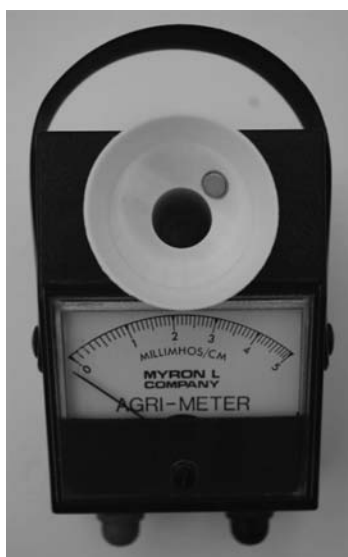
FIGURE 16.7 An electrical conductivity meter.
