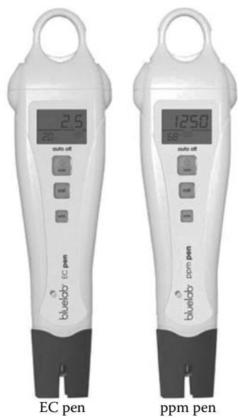
FIGURE 16.8 A “pen” type hand-held electrical conductivity and ppm tester. (Courtesy of BlueLab Corporation Ltd., Tauranga, New Zealand.)
